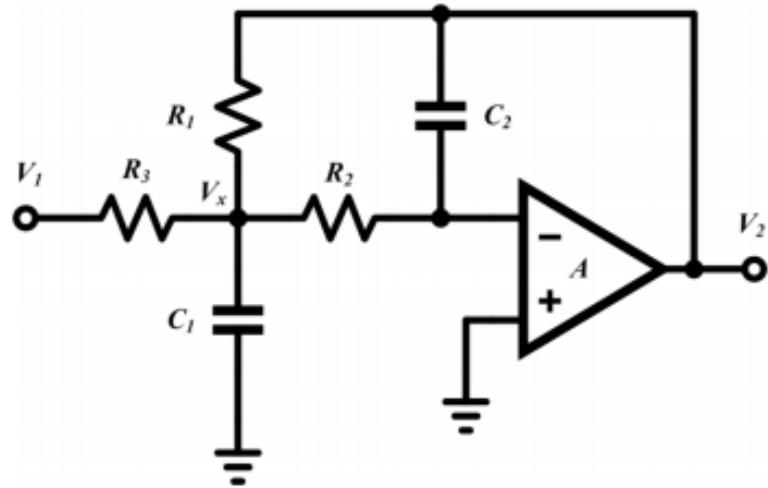
Figure 1 - Rauch Filter Circuit
